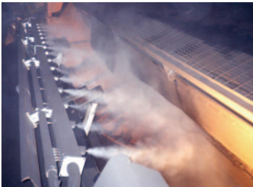
**5. Matched set.** Maximum removal efficiency occurs when the mist droplets are generated at the same rate as the dust particles and applied at the point of dust creation. *Courtesy: Dust Solutions Inc.*
