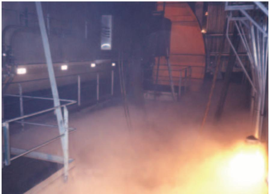
**3. Breathe easy.** Three strategically placed fogging manifolds were placed above the dump pocket grizzly to reduce dust emissions. Courtesy: Dust Solutions Inc.
